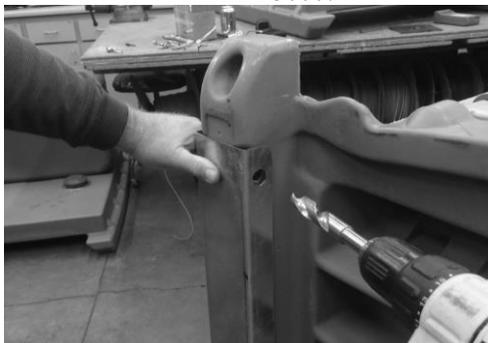
4. Insert the (2) sling threaded ends through the holes in the cradles and base as shown. NOTE: start with one threaded end of sling completely through hole in cradle & base. If other end of sling cannot be inserted by hand completely into hole in cradle & base, try re-drilling hole in cradle & base with 11/16" drill bit.
